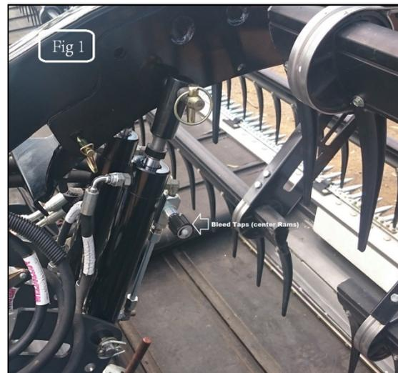
**Fig 1:** Reel Centre Lift Hydraulic Cylinders & Bleed Tap
