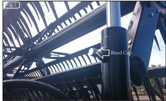
**Fig 2:** Reel Outer Lift Hydraulic Cylinder & Bleed Cap
